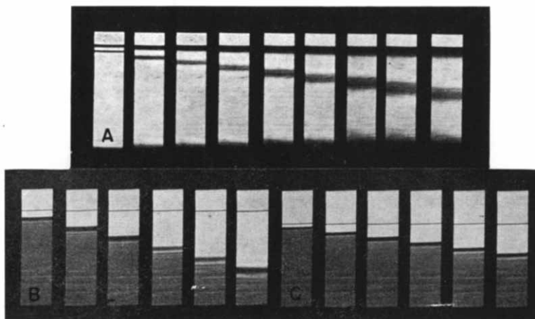
Fig. 1. (a) Schlieren diagram of virus particles sedimenting in dilute plasma (see text); (b) diagram of particles sedimenting in bovine serum albumin solution; and (c) diagram of particles sedimenting in D_2O solution.
